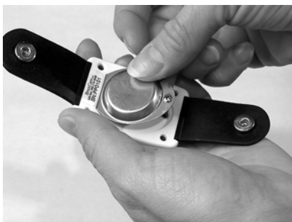
Tuck in tabs first, then tighten screw
