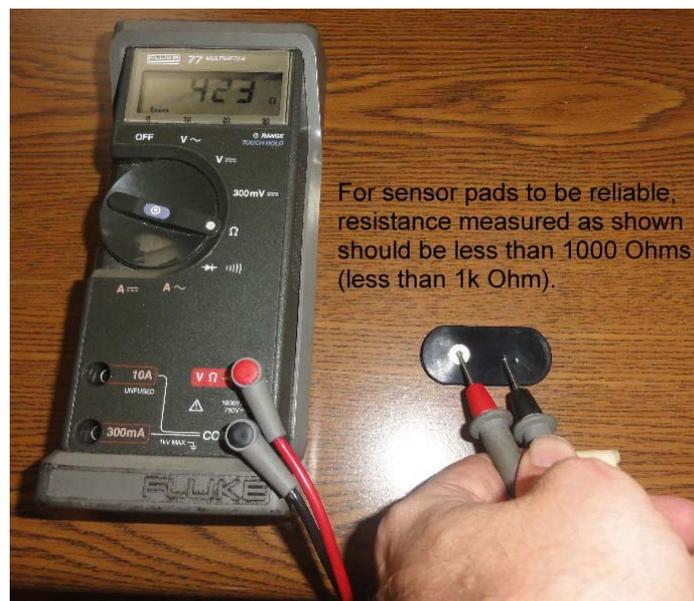
For sensor pads to be reliable, resistance measured as shown should be less than 1000 Ohms (less than 1k Ohm).
